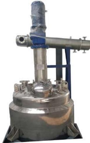
*Double Jacketed Mixing Tank (Reactor Tank)*
