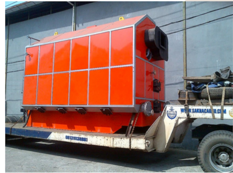
Vertical Water Tube Boiler For Alcohol Plant
